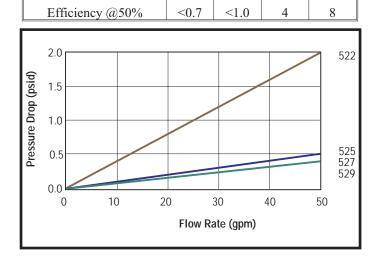
Efficiency: The Series 500 High Performance Filter Bags are rated using a silica test challenge in water at 25 gpm (5.7 cu m/hr). The results reported are typical
